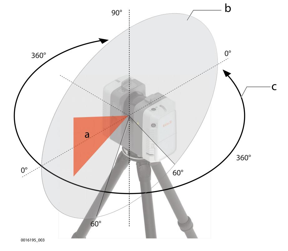
a Laser beamb Vertical laser scanning areac Horizontal laser scanning area
